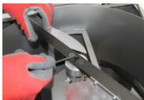
2 Loosen the central screw of the shaft.
