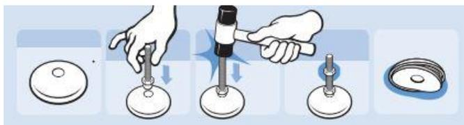
Assemble the short rubber feet in front of the machine and the longer ones on the back. Thus being able to tilt the machine.
